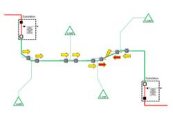
HV sensor system with fault detection and diagnosis technology, that quickly and correctly identifies the faulted transmission line section
